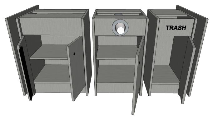
Align all cabinetry in place according to the layout ordered. Bolt end panels and cabinet modules together using the male and female bolts, with the Allen wrench provided in the hardware.
